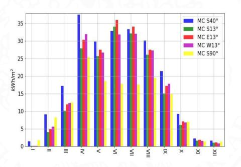
The total generated energy in 2019 by differently orientated panels
