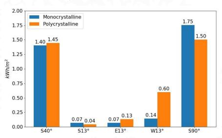
Comparison of the generated energy for PC and MC panels in June 2019
